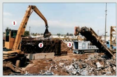
**HOW IT WORKS** First, a crane **1** dumps 47,000 pounds of steel scrap into the Fastek machine **2**. The truck **3** backs up to the machine and is hooked to it. The machine rolls its scrap-containing drawer into the shipping container on the back of the truck, then lowers a steel plate to hold the scrap in while the drawer pulls out. After that the truck **4** drives to port and the container is loaded on a ship to Asia.
